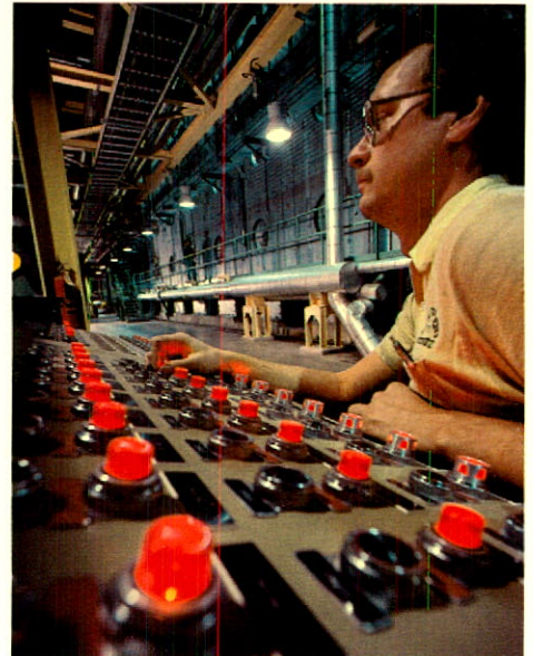
Automatic pulp dryer process control system in the new bleached kraft pulping operation at Espanola, ensuring better quality control and improved operating efficiencies.
