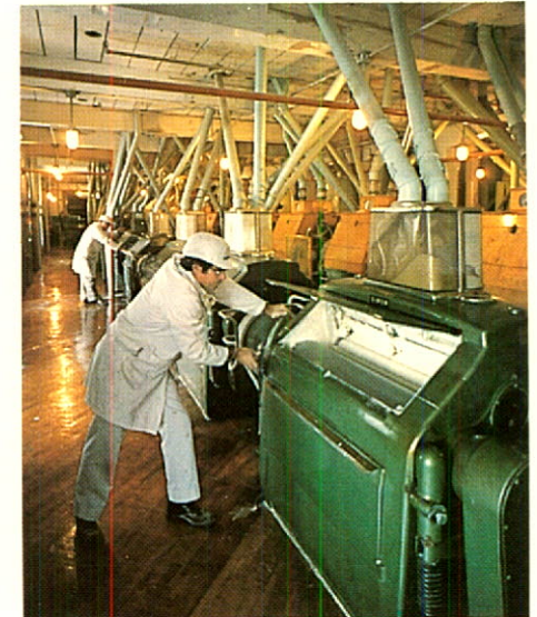
1. Roller mill floor at McCarthy Milling in Streetsville. This illustrates one of the final stages of grinding wheat into flour. 2. New English muffin line in our Kitchener bakery showing muffins coming out of griddle on the way to the cooler. 3. Automated chocolate storage and distribution system being installed in the William Neilson Toronto plant. This system gives the ability to handle a larger range of formulations and distribute them automatically to any point in the plant and measure consumption and storage quantities at any time of day.
