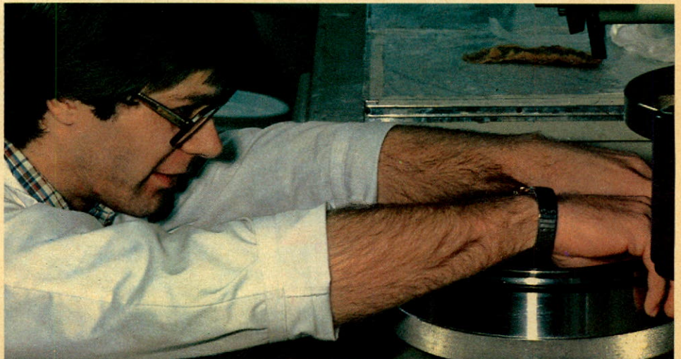
Lab Technician Alain Caron checks pulp strength with P.F.I. mill at Edmundston Lab.
