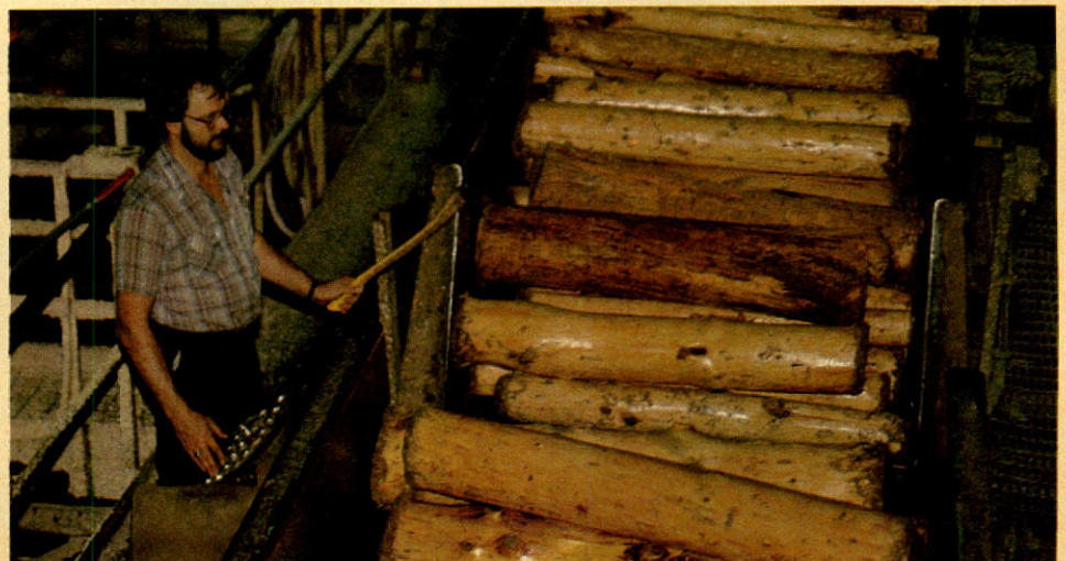
Groundwood Utility Operator Rino Lavoie prepares to charge grinder pocket. Edmundston Groundwood Mill.
