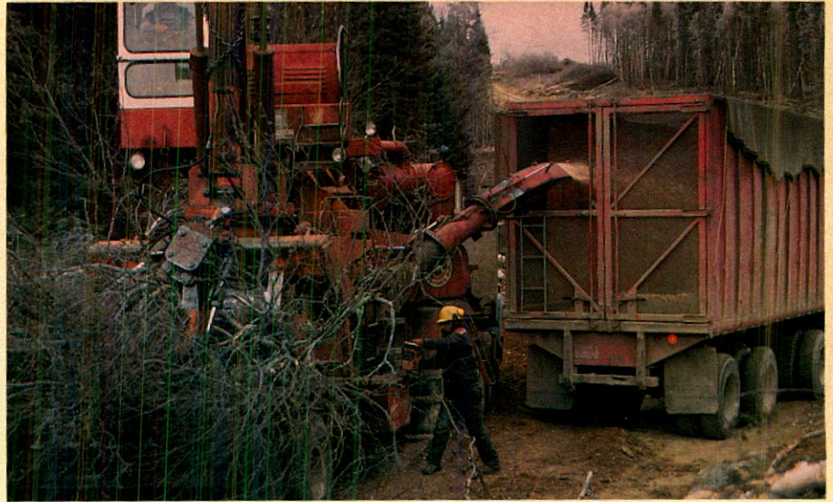
Residual hardwood biomass transformed into chips by a whole-tree chipper on the harvesting site.
