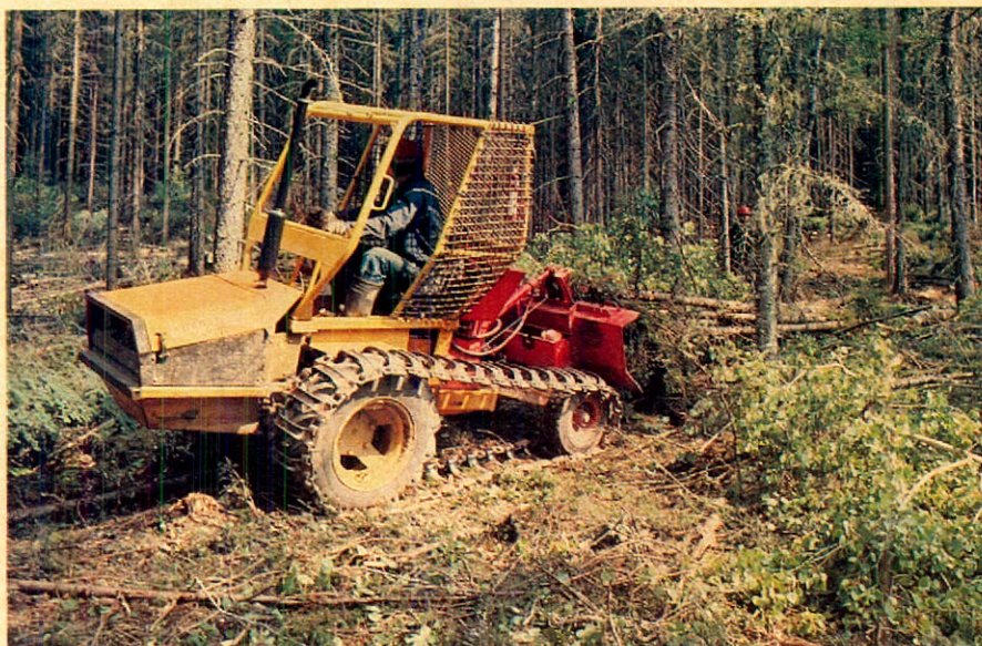
The Krabat, an effective skidder for small woodlot selective cut operations
