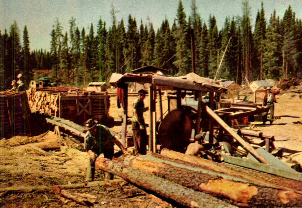
The portable slasher cuts full-length trees rapidly into 4-foot lengths
