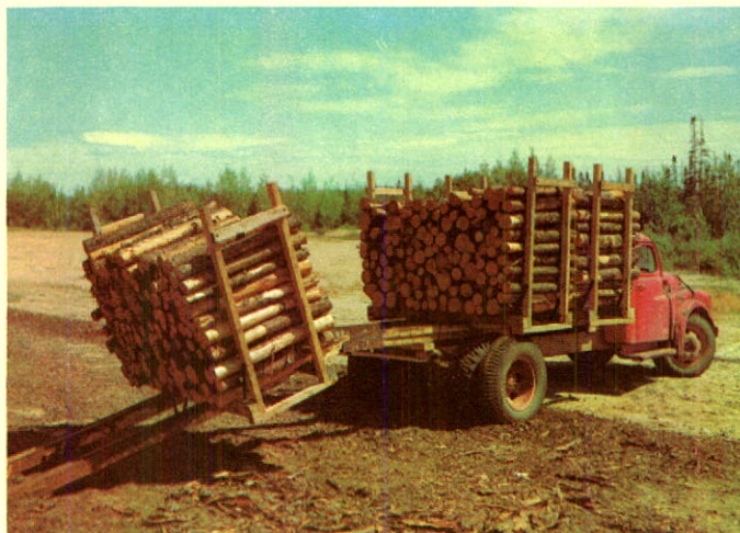
Small pallets are winched in succession onto truck chassis
