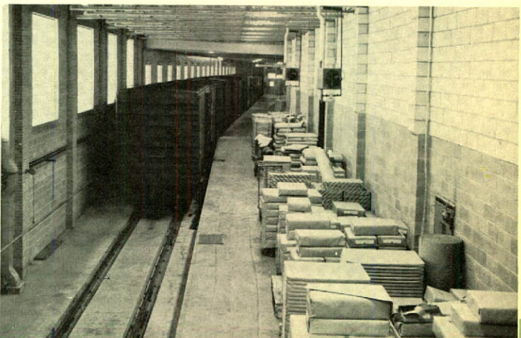
Internal railroad dock protects paper when loading cars, Canada Paper Company, St. Francis Division.
