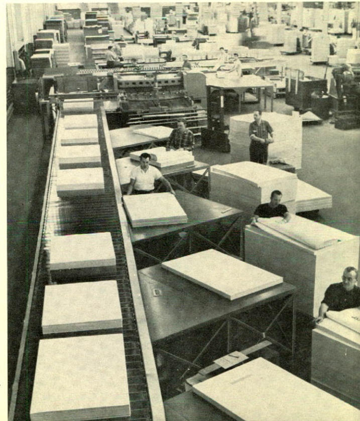
Automatic conveyor at Cornwall Division. Howard Smith Paper Mills, carries counted sheets to paper trimmer.
