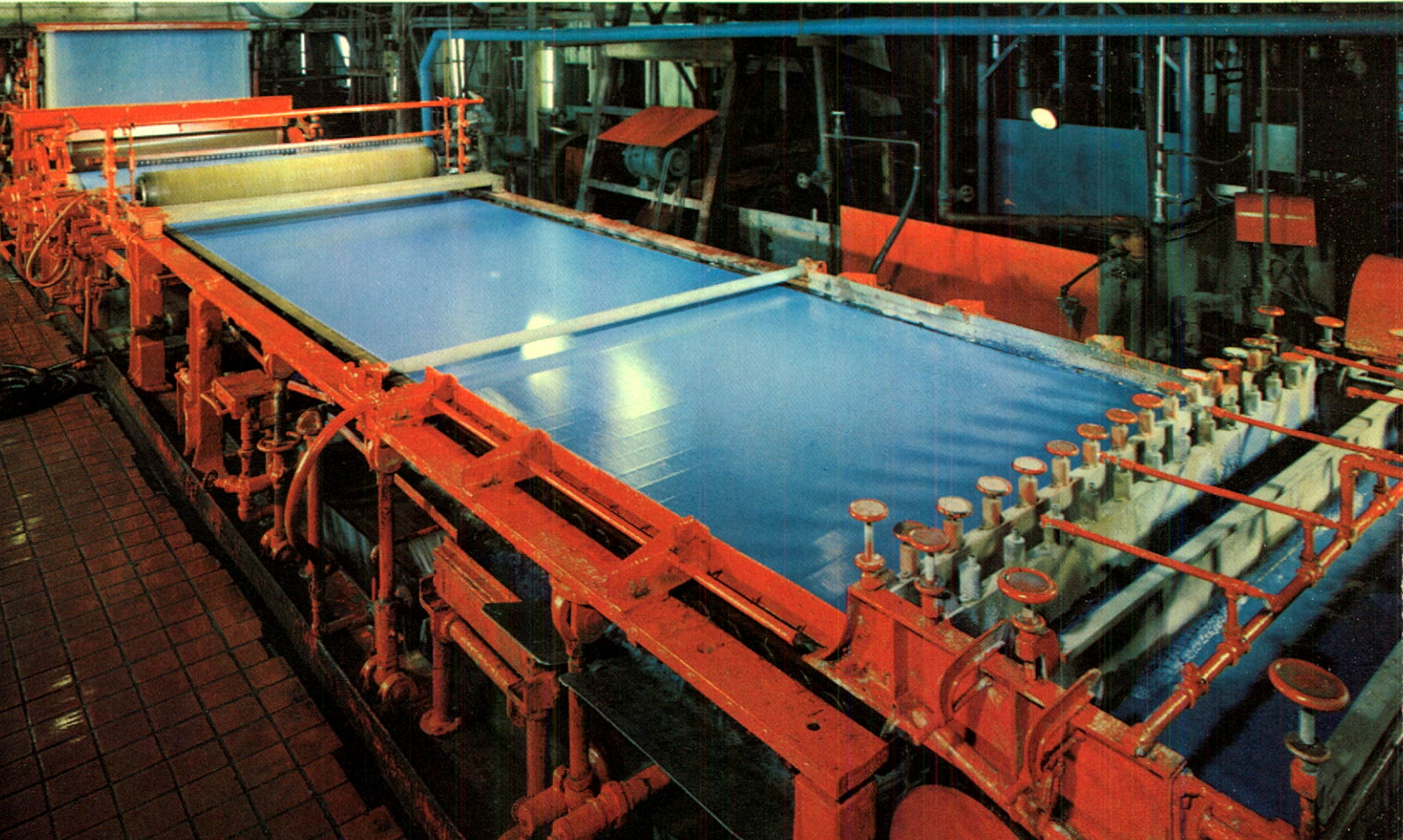
The wet end of the Fourdrinier Paper Machine in the Don Valley Mill. It is designed and equipped to make Cover Papers, Bristols, Tag Stocks, Blotting and other "thick" papers
