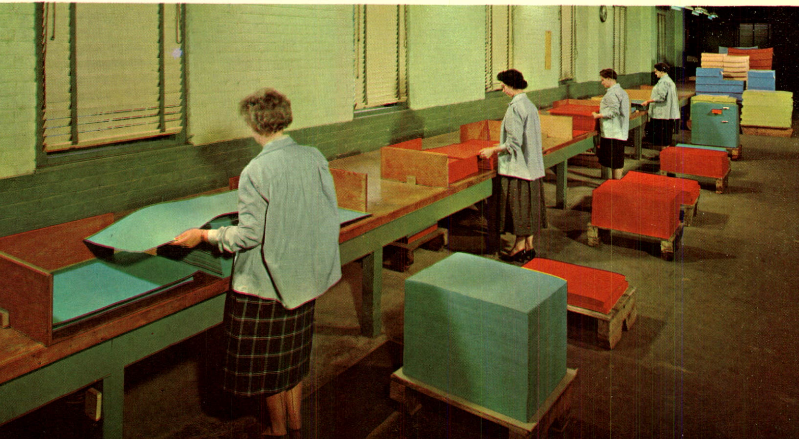
Sheets of Cover Paper are examined on both sides in the Finishing Room at the Don Valley Mill
