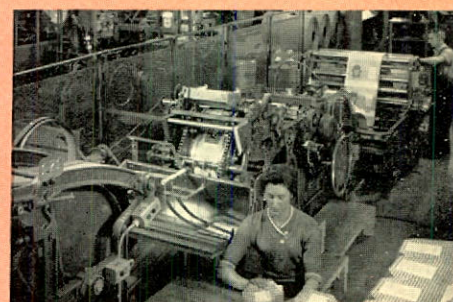
New specialty sack machine installed at the Converted Products Division at Windsor Mills for the manufacture of high grade multiprinted bags.
