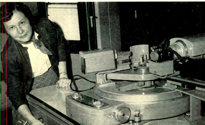
The General Electric X-Ray diffraction and fluorescent equipment recently installed in the Research Department for the chemical identification of trace elements.
