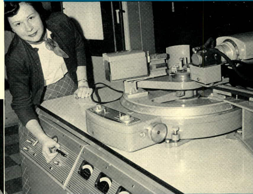
The General Electric X-Ray diffraction and fluorescent equipment recently installed in the Research Department for the chemical identification of trace elements
