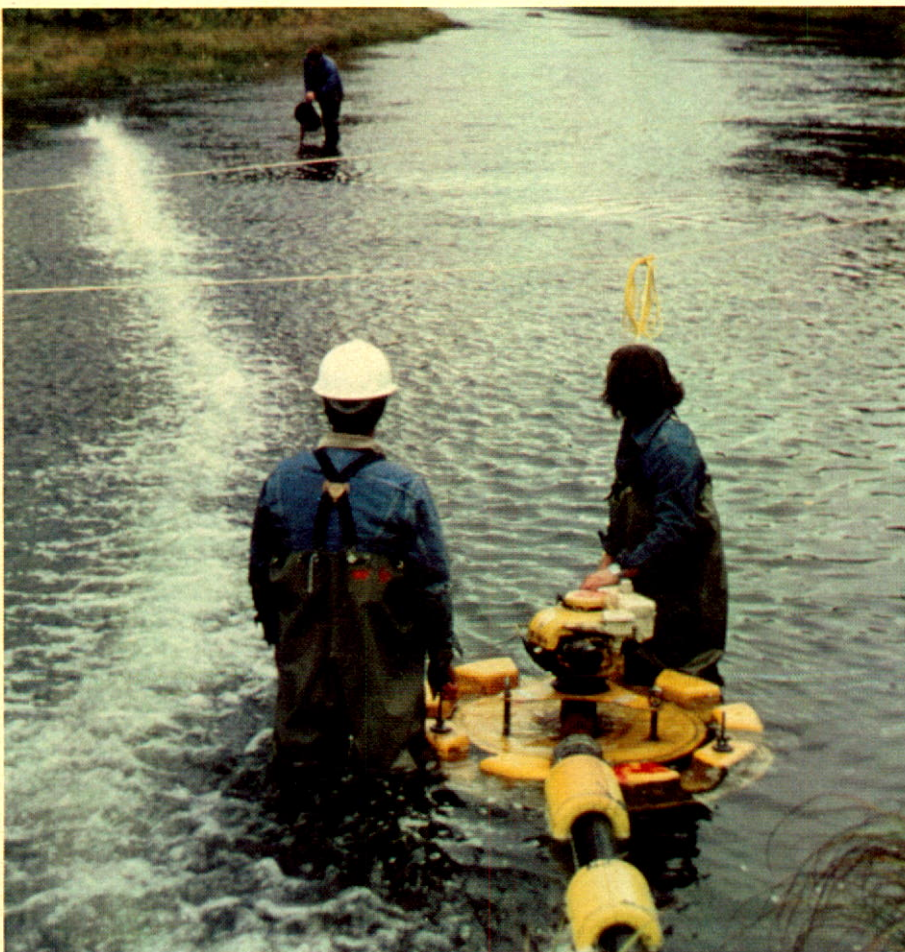
A Company co-ordinated exercise testing the use of air bubbles to contain oil spills.
