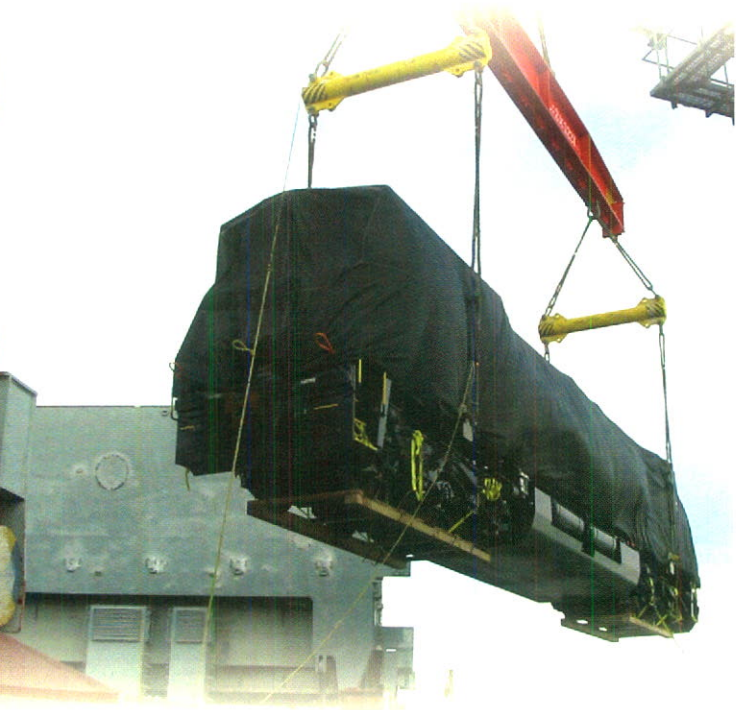
February 2006 - VM/S Hercules lifted 191 metric tons locomotive on the BBC California Vessel
