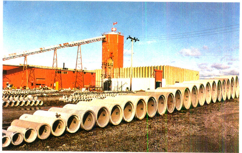
A display of pipe sizes from 6 inches to 12 feet, manufactured at Concrete Pipe Company's Mississauga Plant.
