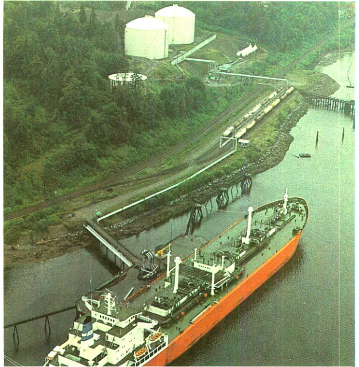
An aerial view of the "YAMAHIDE MARU", a refrigerated Japanese tanker loading liquid propane gas at the Trans Mountain Westridge Terminal. The 30,000 ton ship has been delivering LPG cargoes to Japan from Westridge since October 28, 1966.
