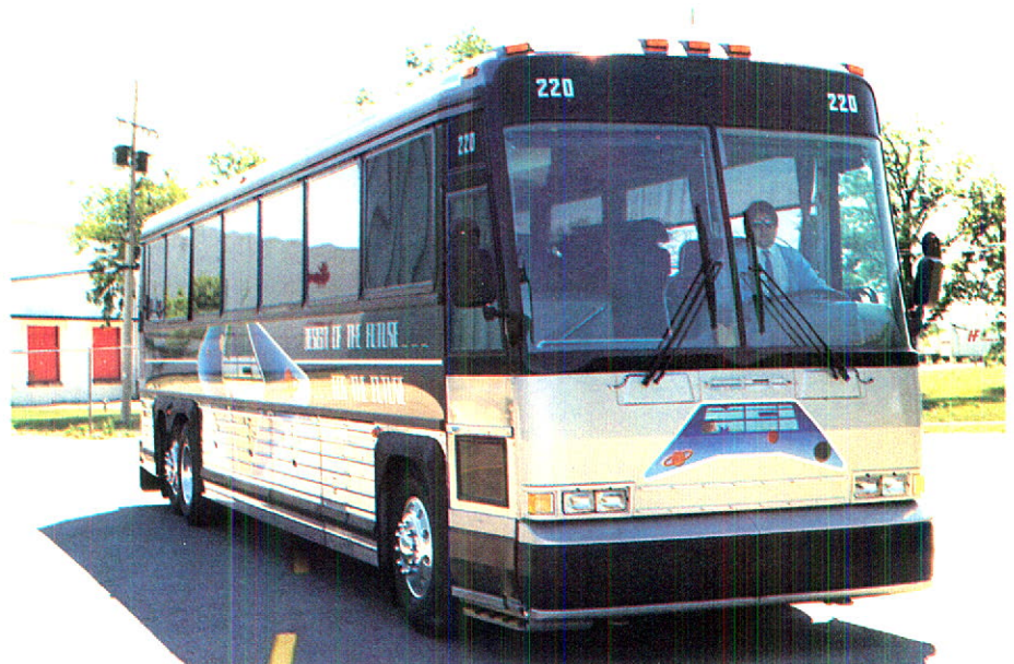
The first MCI 102C3SS tour coach, used as a demonstration model by the Canadian sales division. This model has highly-durable polished stainless steel lower side panels, especially suitable for harsh climatic conditions.
