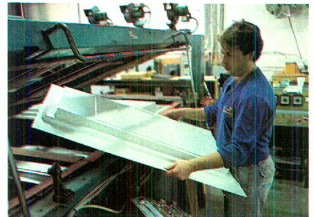
Bob Koerner at Frank Fair Industries removing a finished vacuum-formed fiberglass panel which will become the underside of the parcel rack, housing the passenger reading lamp and air distribution system.
