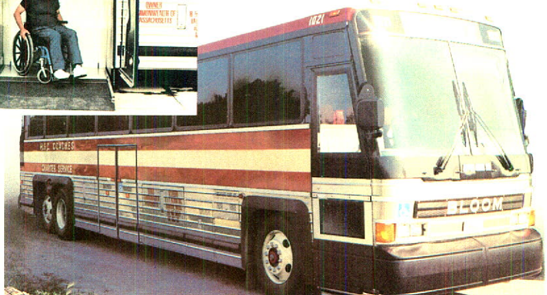
MCI's new generation wheelchair coach; Jay Padden demonstrates the lift.
