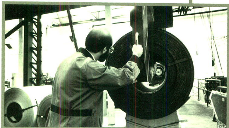
Powered travelling crane indexing steel coil
