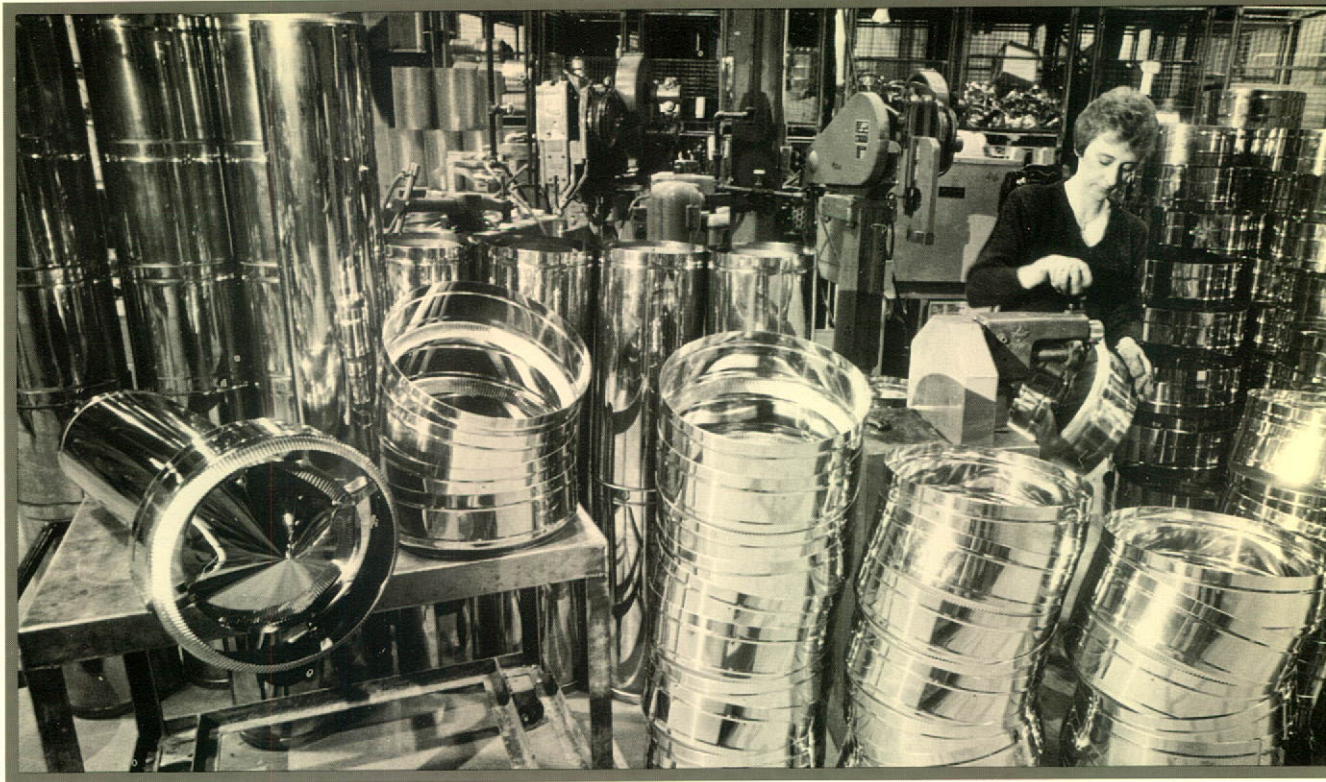
Crimping ring cap components for superchimney
