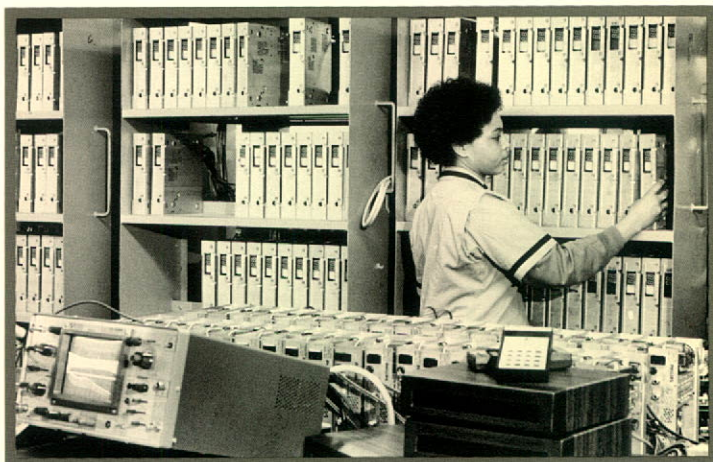
Completed converter assemblies racked for testing in burn-in room
