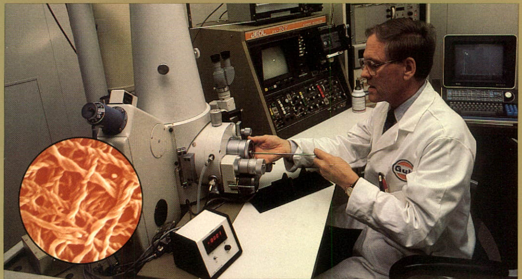
Research chemist Max Hahto studies lithium soap fibres (inset) used in special greases.
