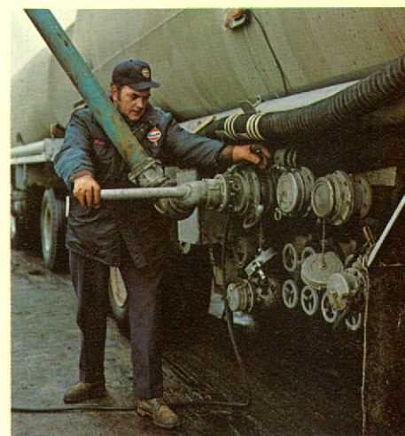
New bottom-loading valves on tankwagons reduce evaporation.
