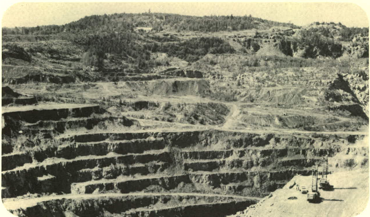
Hogarth Open Pit — stripping benches on hanging wall — main office in background.
