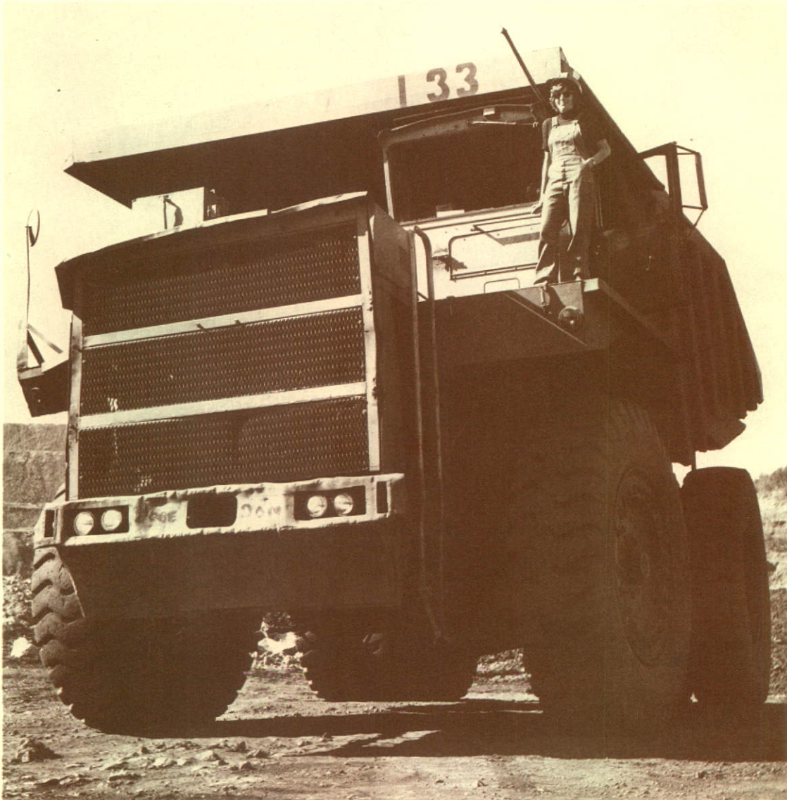
Cheryl Alexiuk, Truck Driver, on a 100-ton Lectra Haul truck in the open pit
