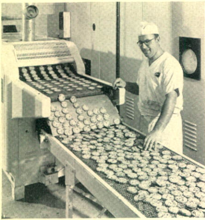
Automatic Cookie Machine mixes, bakes, cooks and packages up to 250 dozen cookies per hour.
