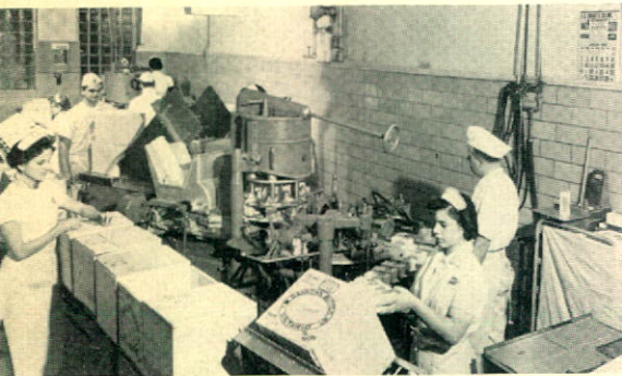
Canada First Grade Creamery butter is automatically cut and packaged under the strictest controlled conditions, at the rate of 50 lbs. per minute.
