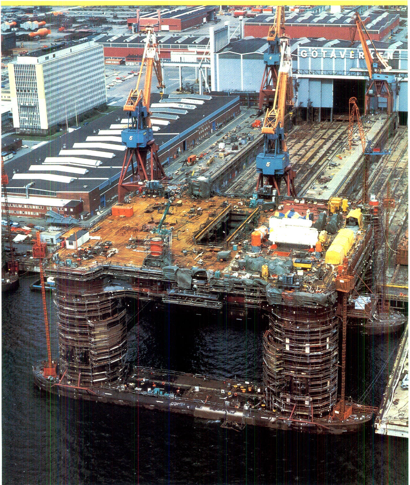
The Floating Production Vessel for the Balmoral field in dry dock at the Götaverken Arendal yard in Sweden prior to completion of construction in 1985. The vessel was being prepared for float-out to a quayside position for installation of production and processing equipment
