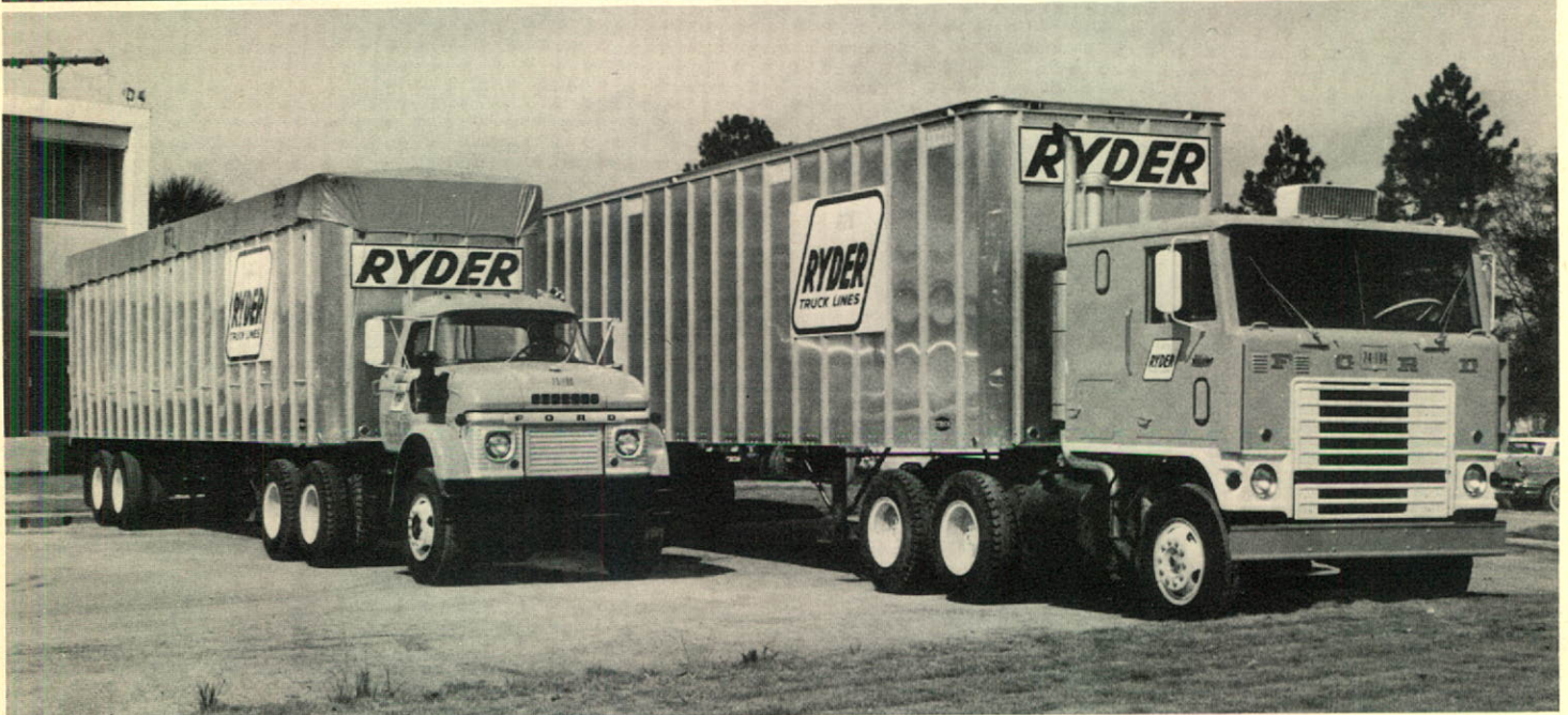
The first of 200 new diesel engine Ford tractors being placed in service by Ryder Truck Lines, Inc. with a new open top Strick trailer is shown with one of the company's new air-conditioned sleeper-cab Ford tractors coupled with a new 45-ft. Strick van.
