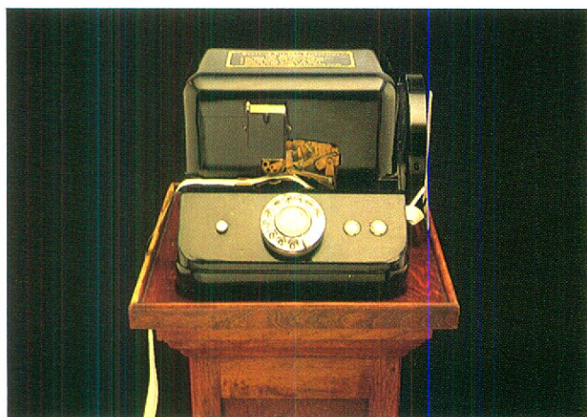
Pictured above is the Dial Ticker which in 1937 was unique to The Toronto Stock Exchange. It was designed for the Exchange by Canadian National Telegraphs and Teleregister Corp. For the first time, a stockbroker could obtain current market information on a specific stock by dialling the appropriate code number.
