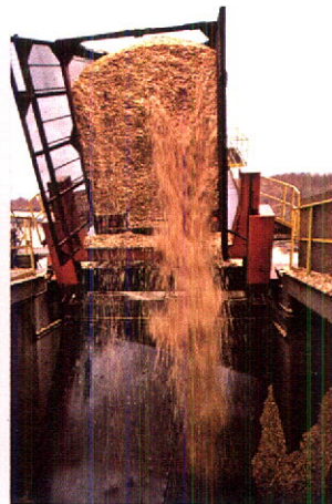
Hydraulic dump ramp tilts tractor and trailer.
