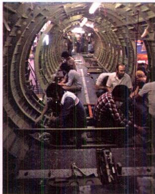
Sub frames are assembled to form a Dash 7 fuselage.
