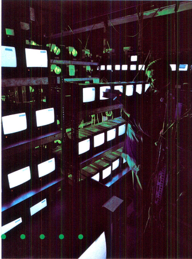
Quality Assurance technician measures the light output of a video display unit. Equipment like this is life-tested by running sixteen to twenty hours a day for up to two years.
