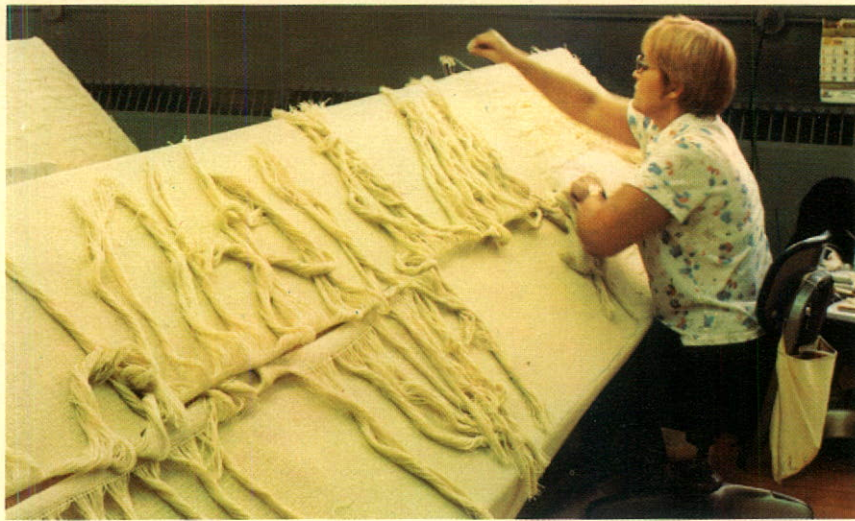
Seaming a paper machine felt.
