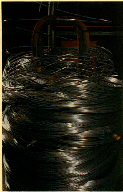
Galvanized wire being coiled.
