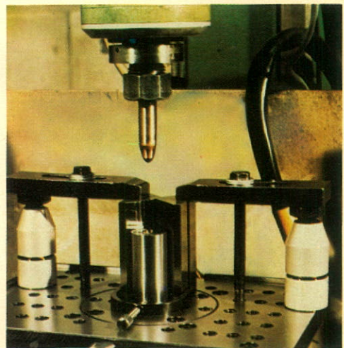
New "cutting tool" forms carbide dies.
