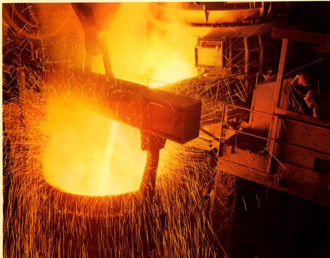
Final materials are added while tapping the heat.
