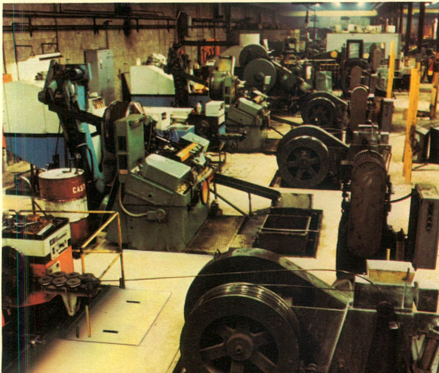
Part of a high speed boltmaker line.
