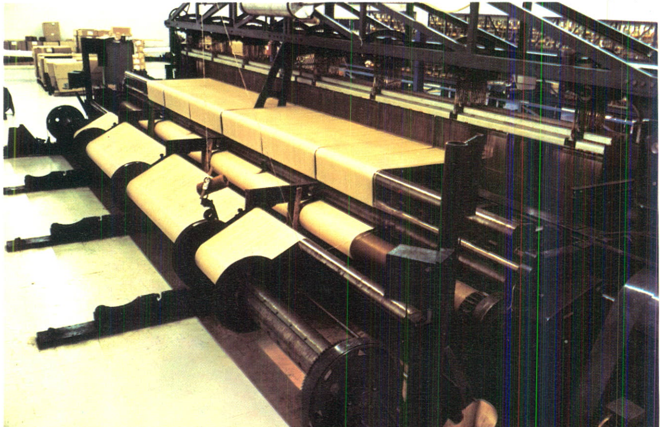
Loom for production of wet felt.
