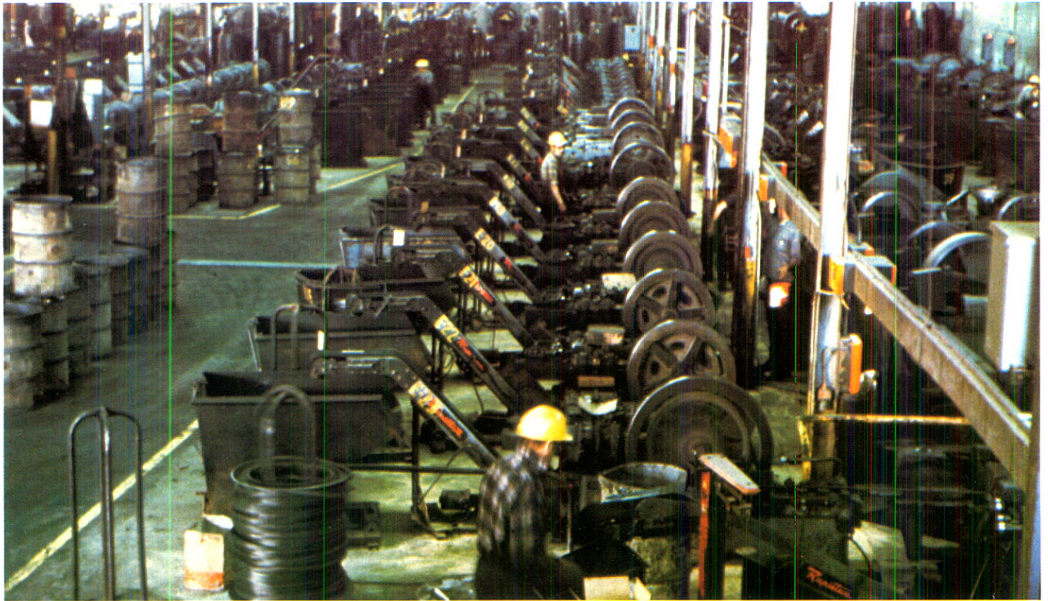
▲ This is one of several banks of automated nail makers.
