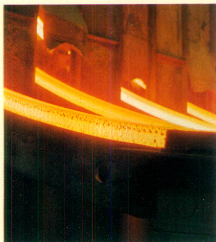
▲ Four strand continuous casting
