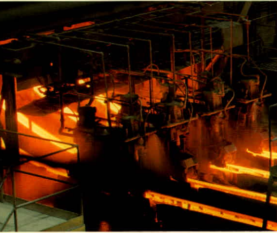
4-strand continuous caster at L'Original.
