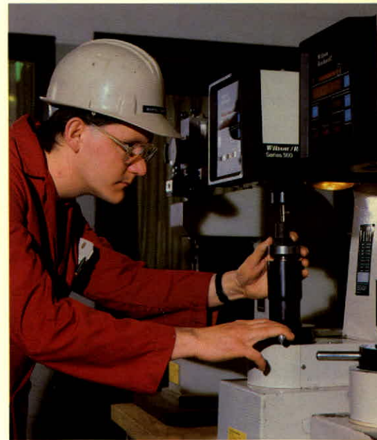
A cold forged bolt passes one of the many quality control tests required before shipment.
