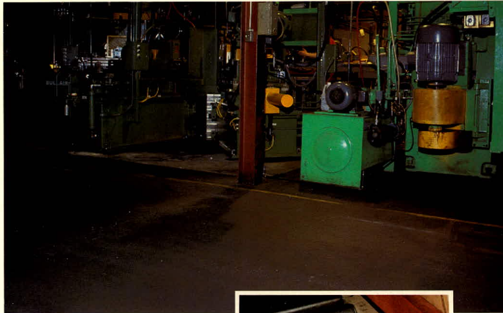
Newly installed rotary transfer system for the machining of engine water pumps at Ingersoll.
