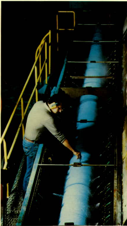
C-900 plastic water pressure pipe being tested prior to shipment.
