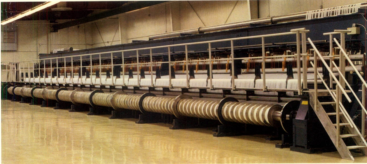
Niagara Lockport's 30 meter loom can weave wet felts for the world's largest paper machines.
