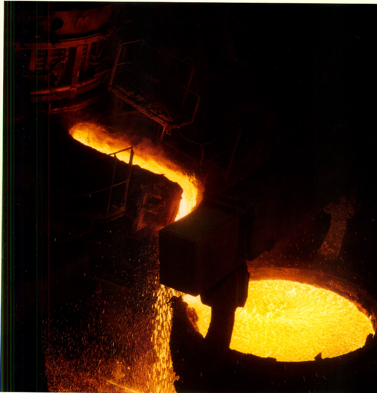
Molten steel is tapped from a furnace into a ladle at L'Original.
