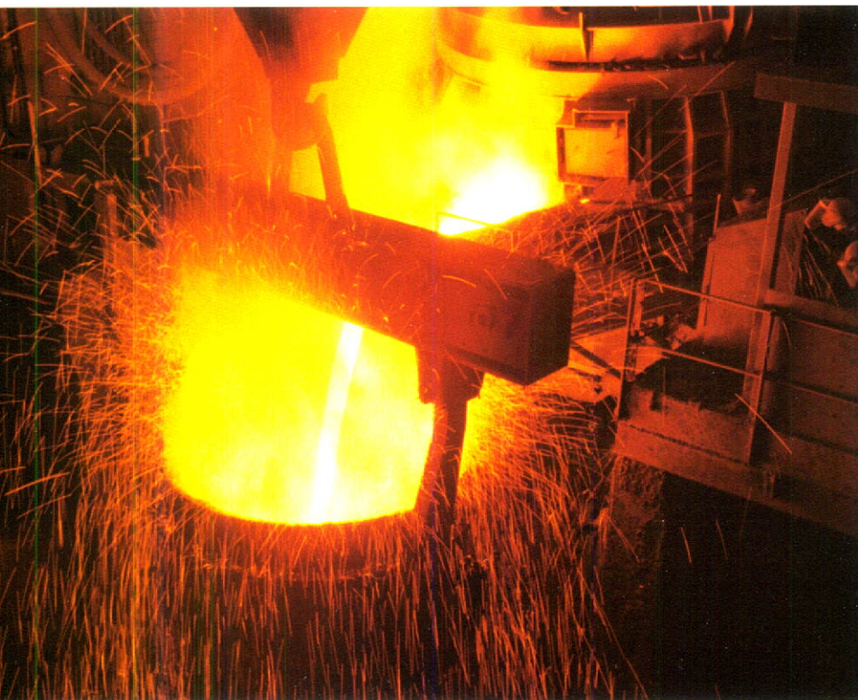
Tapping the electric arc furnace.
