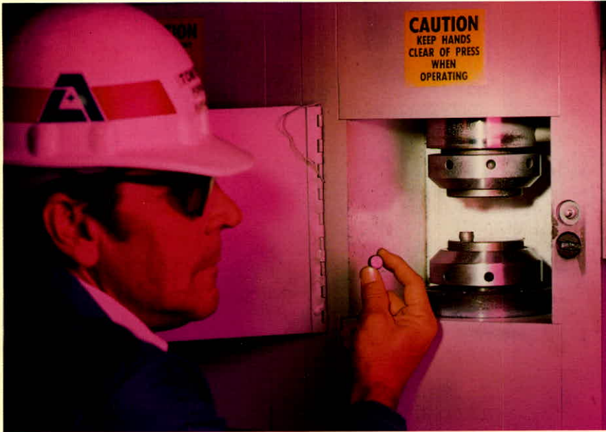
Upset tester at Atlantic Steel used to ensure integrity of high carbon and cold heading quality steel.
