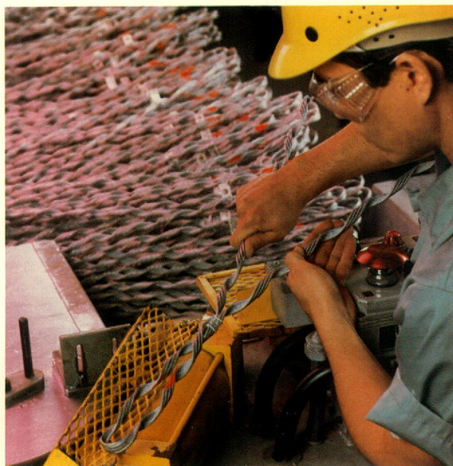
Florida Wire and Cable's galvanized steel grips for use in the electrical power and communications industry.
