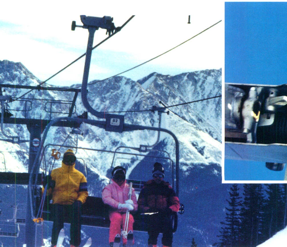
This state-of-the-art high speed detachable chair ski lift designed and installed by Doppelmeyer Lifts operates with wire ropes manufactured by Wrights Canadian Ropes at the 1988 Olympic ski site.
