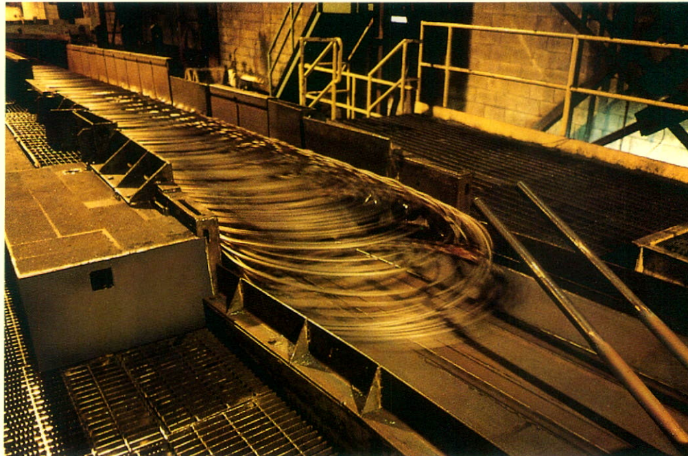
Hot rolled wire rods complete controlled cooling at L'Orignal, Ontario.
