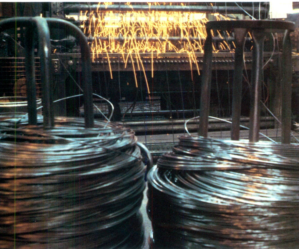
High capacity welded wire fabric production at Baltimore.
