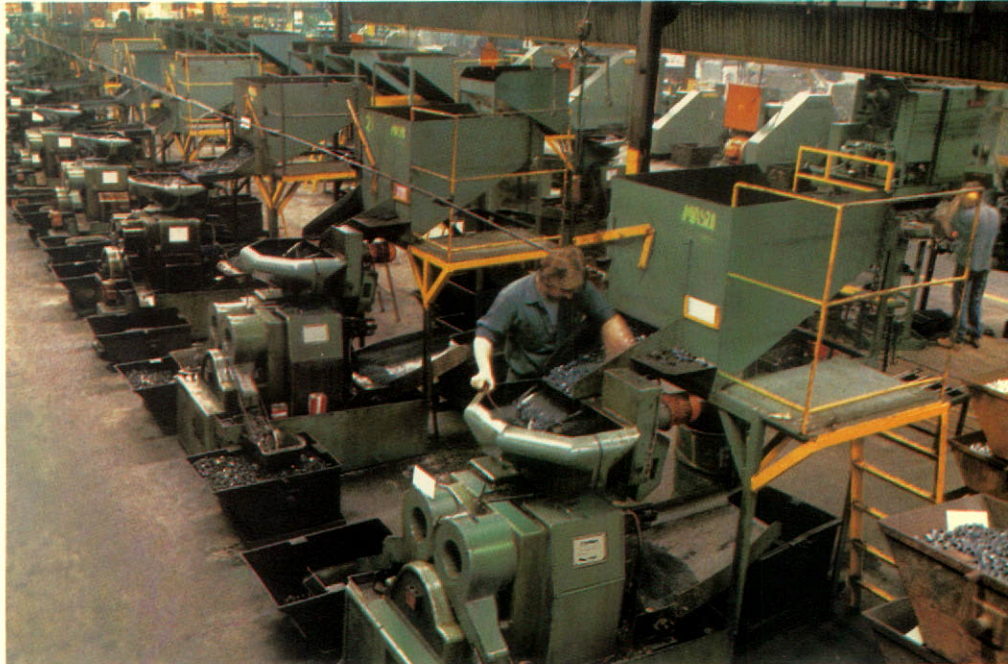
Part of Federal Bolt and Nut's line of high speed bolt makers.
