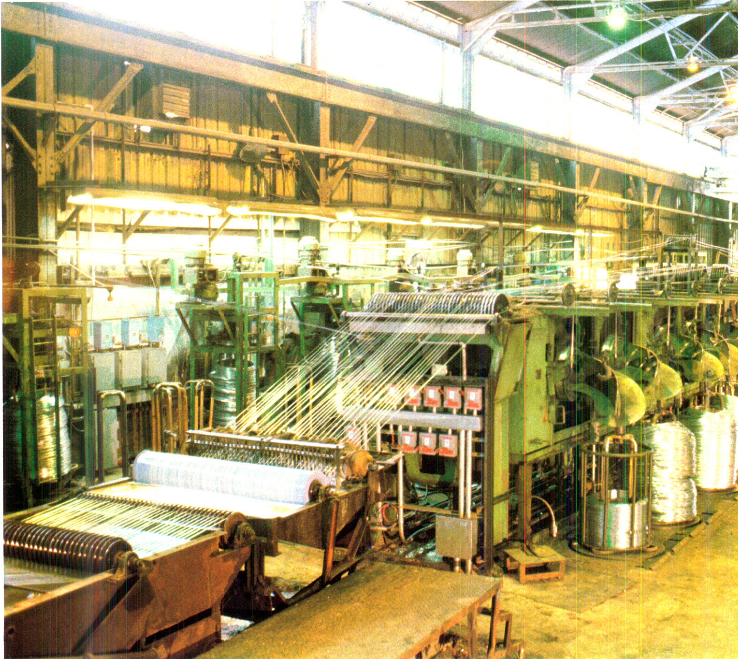
▲ High-speed strand galvanizing line at Atlanta.
