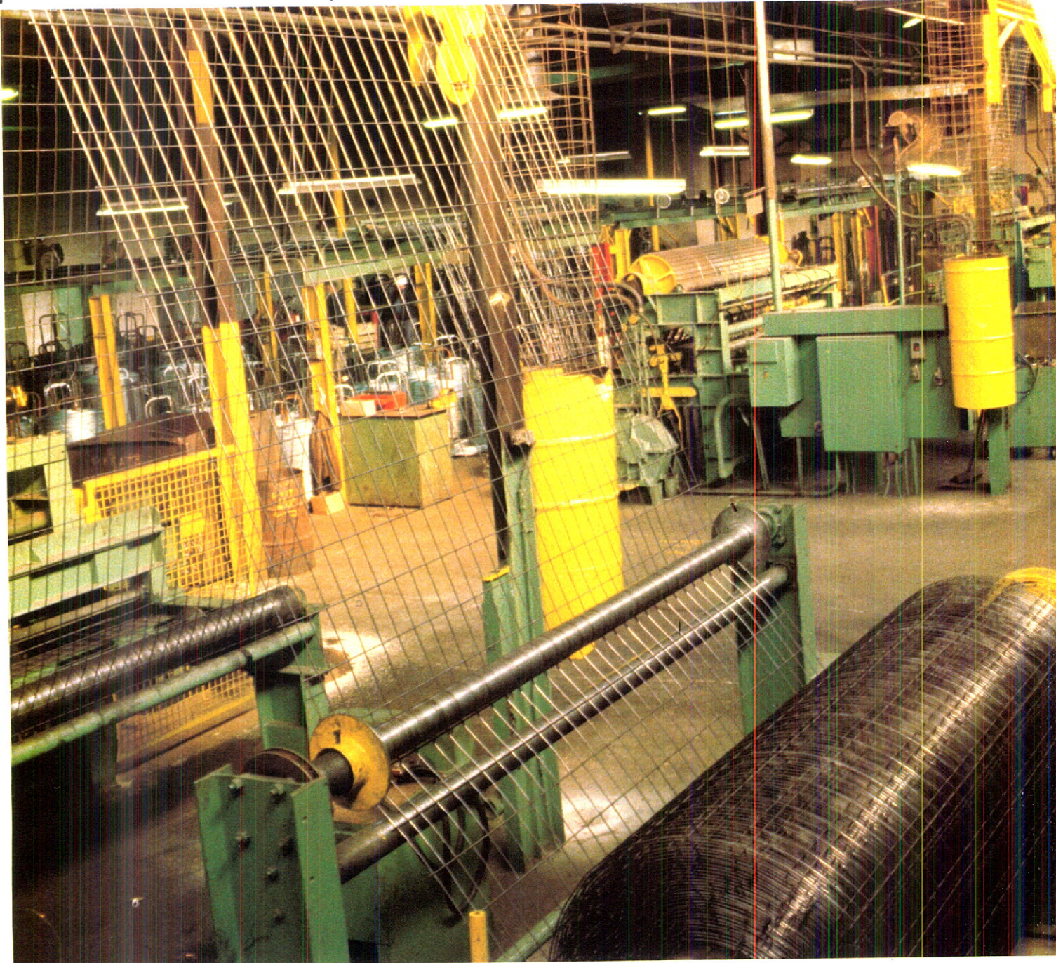
▲ Welded wire fabric machines in operation at National Wire.
