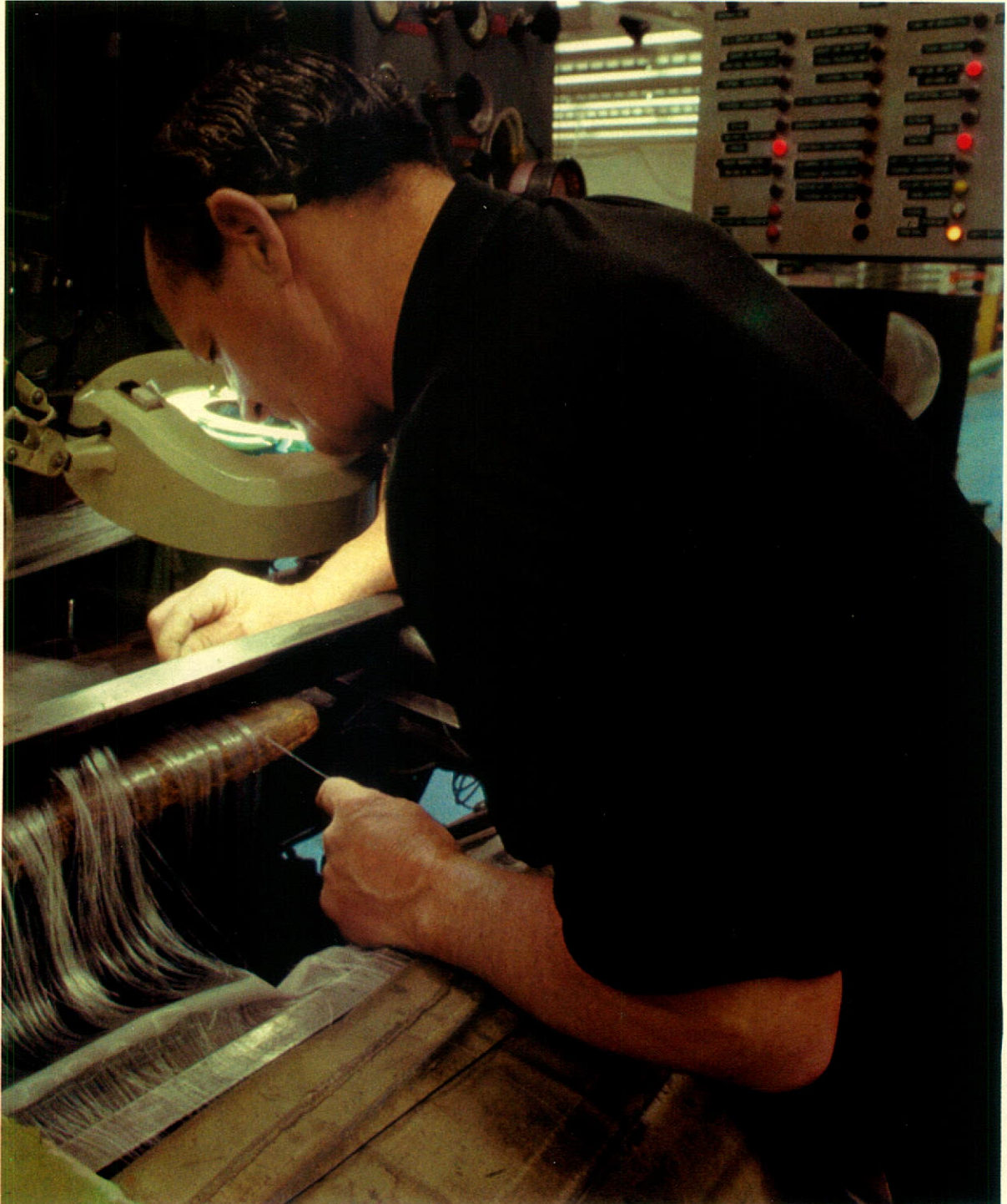
▲ Loom set-up for paper machine fabrics is a meticulous process as each fabric is custom designed for the machine on which it is used.
