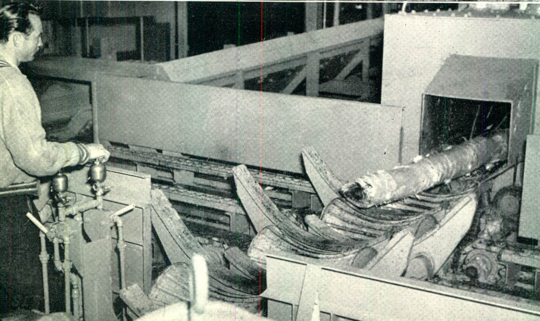
Salvage Wood Passing Through Small Hydraulic Barker
