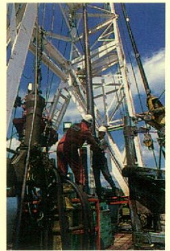
Roughnecks running surface casing in the Caroline area of Alberta.
