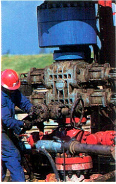
Righand hooking up a blowout preventer.
