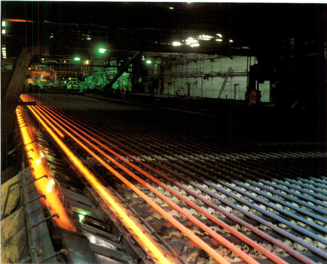
The cooling bed of the new mill moving hot rolled steel in straight lengths for air cooling. The rolling mill is in the background.
