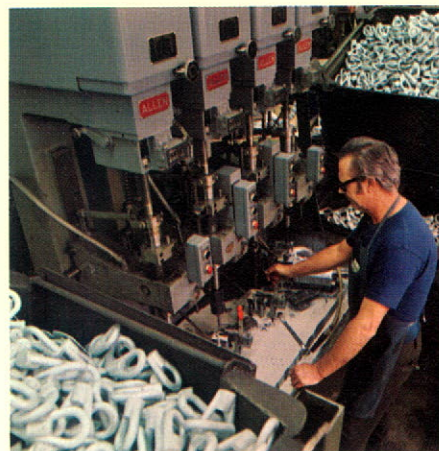
Left: Eye nuts are being drilled and tapped on a Multiple Spindle Drill which allows the operator to perform four operations simultaneously.
