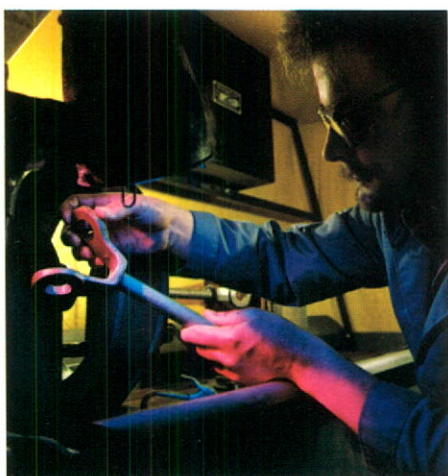
New Magnaflux Testing equipment is used to examine a clevis fitting. This machine uses electromagnetism to identify possible defects in forgings and castings.
