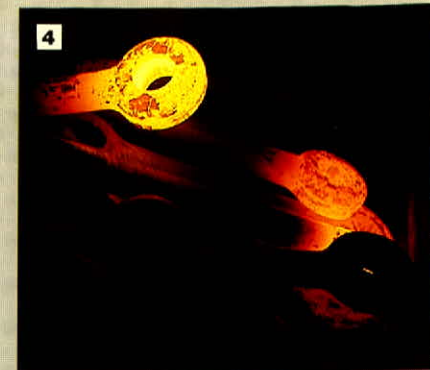
4. Hot forged shackle used in transmission line construction.
