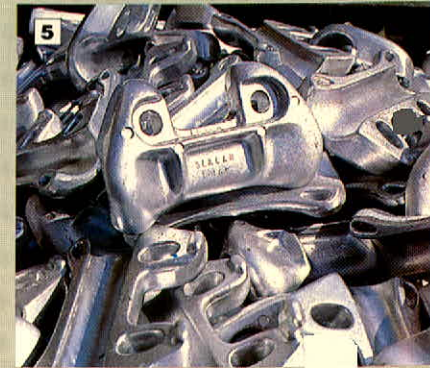
5. Aluminum cast suspension clamp components for support of transmission line conductors.
