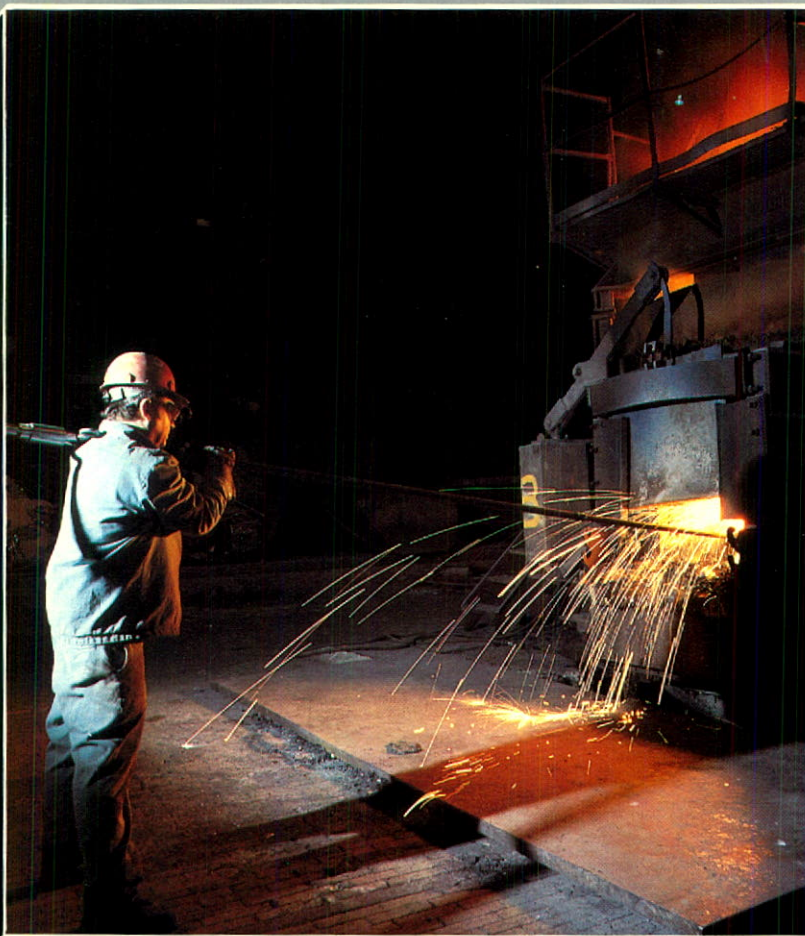
Oxygen lancing for decarburization and productivity improvement during the electric arc melting of stainless steel.
