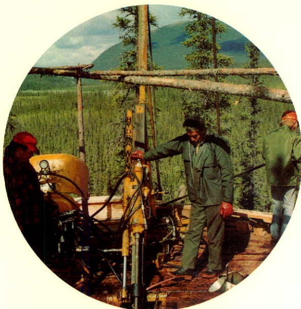
Hydra-Wink Badger diamond core drill in operation, Rusty Springs, Yukon.
