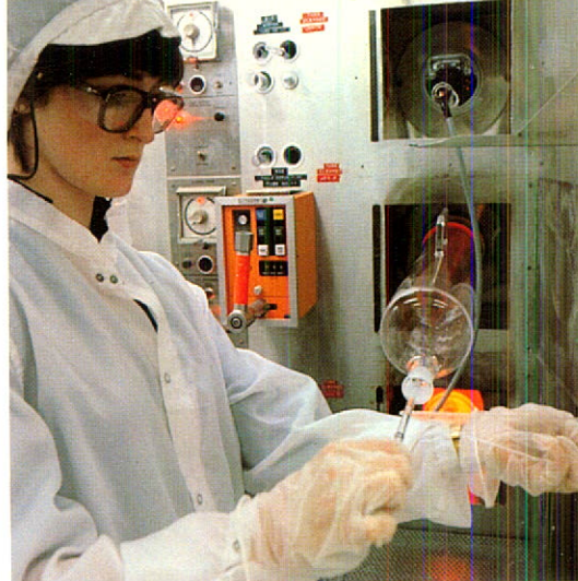
Silicon wafers are inserted into a diffusion furnace. This is a part of the production for large-scale-integrated circuits manufactured by Northern Telecom’s Semiconductor Components Group.
