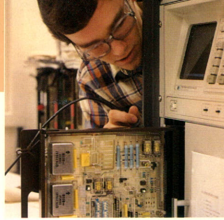
A technologist inspects a long-distance (trunk) circuit pack for a DMS-200 switch produced in Northern Telecom Canada's Calgary, Alberta digital switching manufacturing plant.
