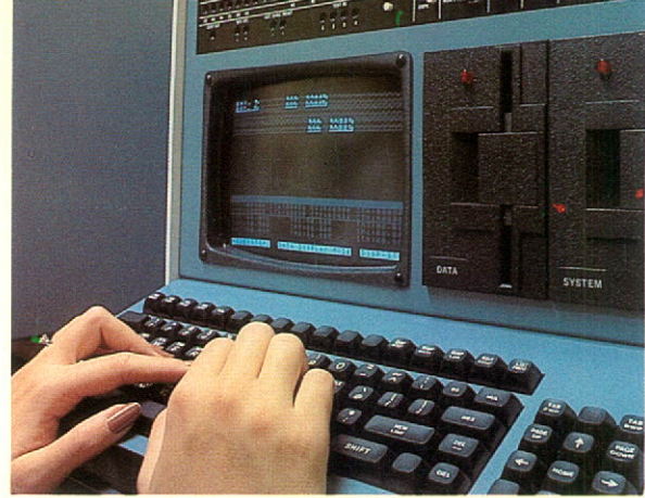
Data test systems produced by Spectron can display data as it is transmitted and received so that hardware or software problems may be identified and analyzed.
