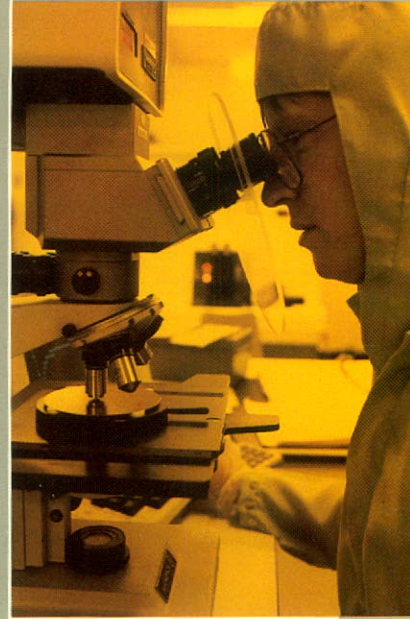
During the wafer fabrication process, a process operator inspects LSIs for proper line width.
