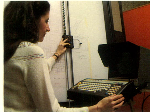
SCG technician uses plotter to enter an integrated circuit design into a computer.
