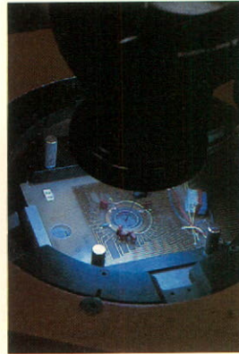
In the probe test of completed silicon wafers, defective circuits on the wafer are defaced by an ink blot from the needle.
