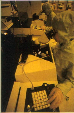
Inspecting the photo resist pattern on wafers prior to the etching process, an operator can sort out bad wafers for reprocessing.
