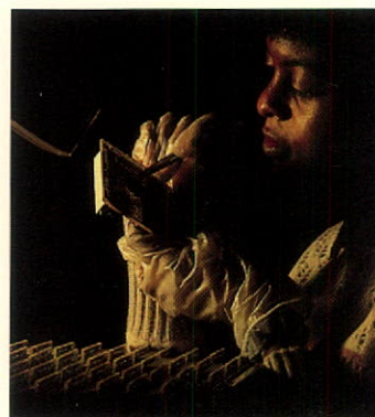
Bernice Sams performs quality inspection of DMS telephone line cards after surface mounting of components has been completed.
