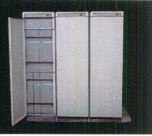
The Meridian DV-1 Data Voice System's computing capabilities are contained in easily expandable cabinets joined by a 20 mbps communications link for data and a 20 mbps line for voice.
