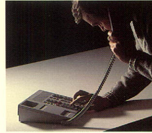
The M2000 series of digital terminals includes the M2112 and M2018 with 12 and 18 programmable keys, respectively.
