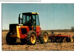
Versatile's Model 256 tractor is a breakthrough in concept, design and manufacture. Its features include articulated steering, hydrostatic drive and a powerful 84 PTO (100 HP) capability.
