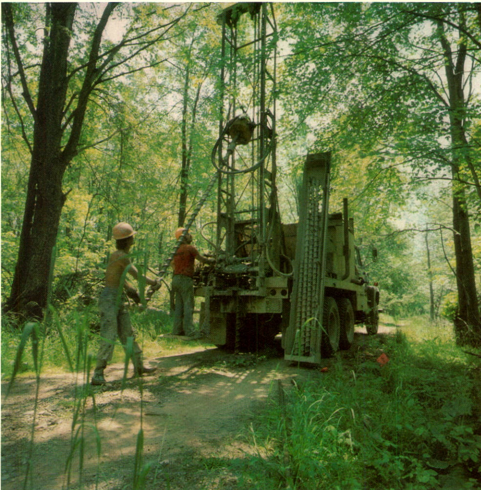
A drill extension being positioned during seismic exploration work in the search for oil and natural gas in southwest Ontario.
