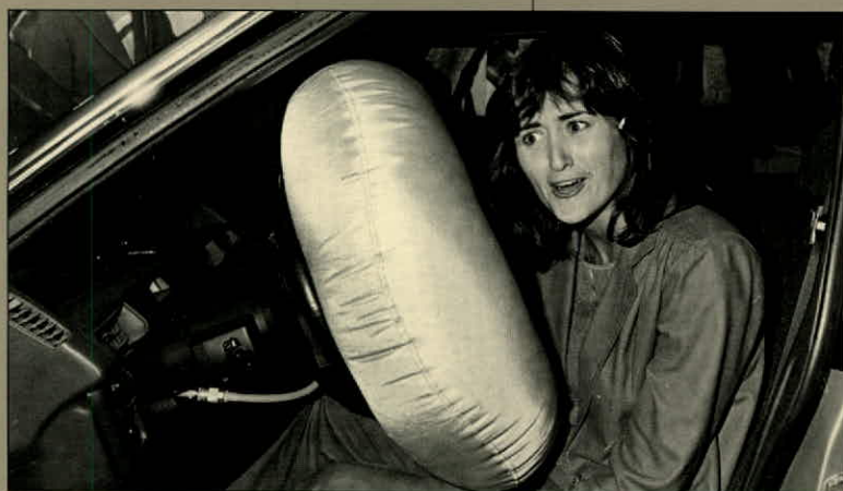
Airbag demonstrations by ICBC surprise participants and amuse onlookers, but airbags have been proven effective in providing almost total upper body protection in vehicle collisions. Airbags are computer-controlled and deliver immediate, automatic protection on impact. The bag balloons from the steering wheel, filling with nitrogen gas. The entire operation takes a twenty-fifth of a second.
