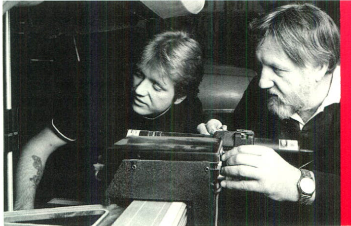
Jack McElree, owner of Ramp Body and Fender Works Ltd. at Nelson, works closely with ICBC personnel and is always proud to demonstrate his high tech Chart Combe Frame Straightener; the only one in the Kootenays. Classified as a triscan laser measuring system, it quickly straightens the frame and structure of unibody vehicles with total accuracy. "It's made working a lot more fun," says Jack.
