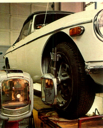
Following an accident, wheel misalignment is common in unitized car bodies because of the impact being distributed throughout the entire car.
