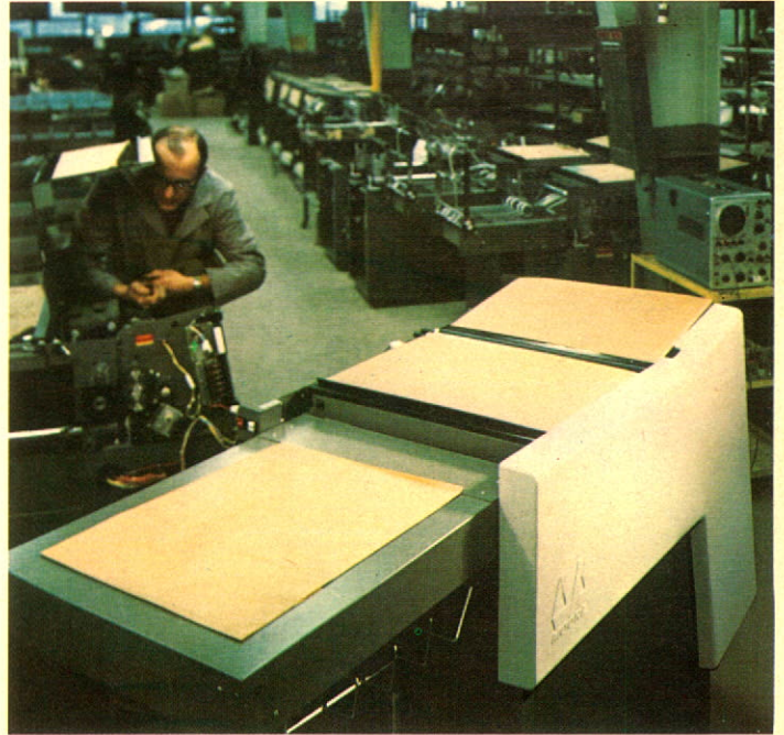
The Machinery and Business Equipment Division provides support for the sale of Moore products by manufacturing forms handling equipment designed to help customers handle such tasks as slitting, imprinting and detaching forms quickly and efficiently. A 3600 Series Forms Processor is shown here in the final stage of production at the Moore plant in Dover, New Hampshire.
