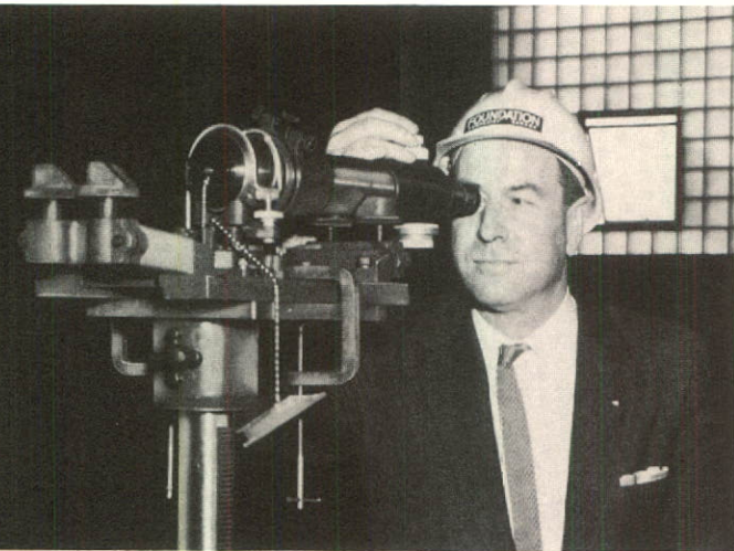
Foundation's optical method of alignment ensures maximum efficiency of mechanical installations.
